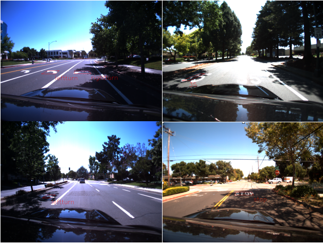
Fig. 3. Examples of detected road markings in shadow regions under various lighting conditions.
