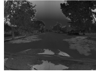
Fig. 4. An example image of the ratio between blue and red channel of an outdoor daytime scene. Note that the ratios are higher (image is brighter) in shadowed areas.
