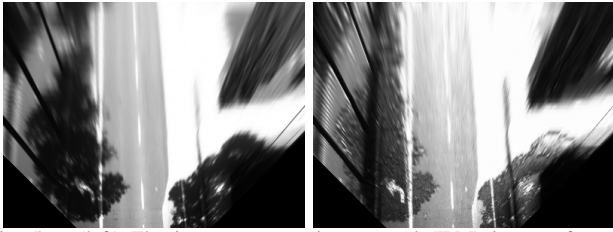
Fig. 5. (left) The inverse perspective mapped (IPM) image of a road marking in shadow region; (right) The boosted IPM image.
