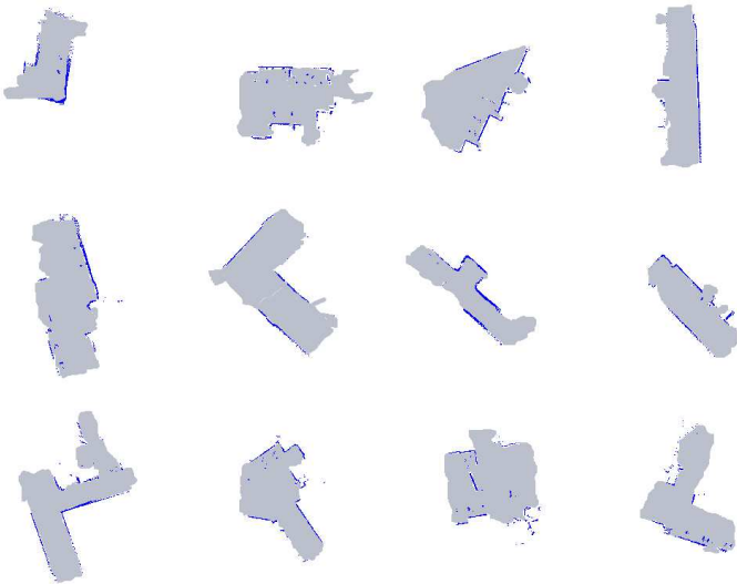
Fig. 1. Scan measurements, obtained by concatenating scans from around landmark locations, used by the RBPF algorithm.
