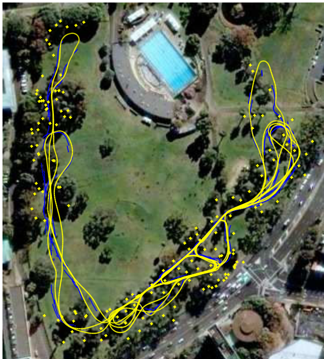
Figure 6: Optimized map of the full Victoria Park sequence. Solving the complete problem after every step takes less than 2 minutes on a laptop for known correspondences. The trajectory and landmarks are shown in yellow (light), manually overlaid on an aerial image for reference. Differential GPS was not used in obtaining the results, but is shown in blue (dark) where available. Note that in many places GPS is not available.
