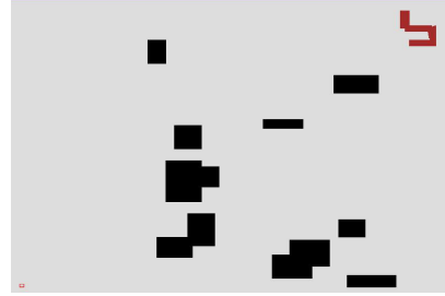
Fig. 6. Randomly generated terrain with a four-link robot at the start location (upper-right corner) and a small square at the goal location (lower-left corner)
