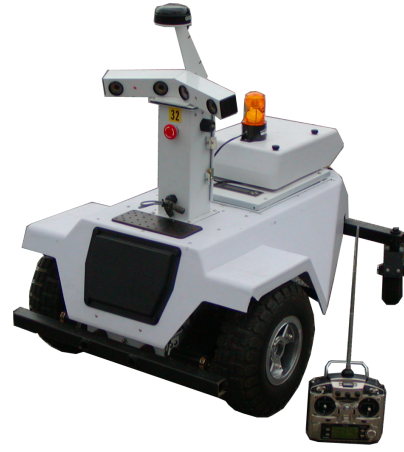
Fig. 5. The LAGR robot with two stereo camera pairs and a GPS antenna on top used in the experiments.
