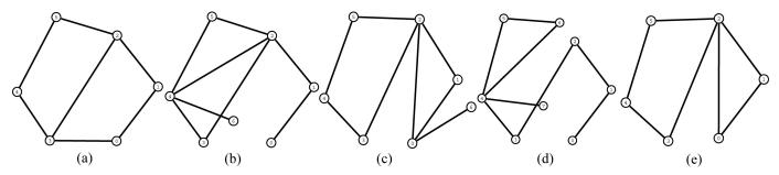
Fig. 14. Topologies with highest posterior probability mass for the second experiment using odometry *and* appearance (a) The ground truth topology receives 94% of the probability mass while (b), (c), (d) and (e) receive 3.2%, 1.2%, 0.3% and 0.3% of the probability mass respectively.
