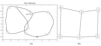
Fig. 9. (a) Raw odometry (in meters) and (b) Ground truth topology from the first experiment involving 9 observations
