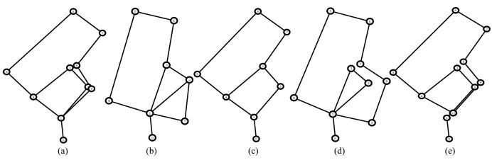
Fig. 17. Topologies with highest posterior probability mass for the third experiment using only odometry. (a) receives 43% of the probability mass while (b), (c), (d) and (e) receive 14%, 7.3%, 3.9% and 2.8% of the probability mass respectively. The ground truth topology is (c).
