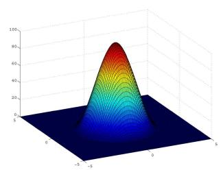
Fig. 7. Cubic penalty function (in this case, with a threshold distance of 3 meters) used in the prior over landmark density
