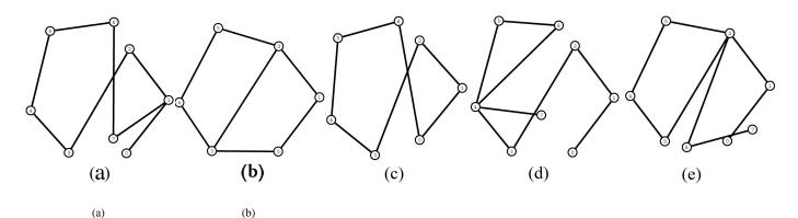
Fig. 13. The topologies with highest posterior probability mass for the second experiment using only odometry (a) an incorrect topology receives 91% of the probability mass while the ground truth topology (b) receives 6%, (c), (d) and (e) receive 0.9%, 0.8% and 0.7% respectively.
