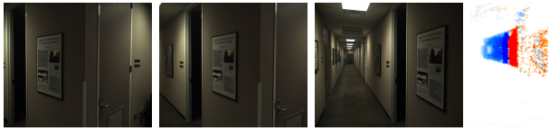
Fig. 11. Input images showing the hallway junction. The floor and ceiling are not observed in some region in the junction. Also the wall on the opposite side is not observed. The last image shows a vertical slice of the occupancy grid. The floor, ceiling and left wall are missing only the right wall is shown in red, which means a positive weight.
