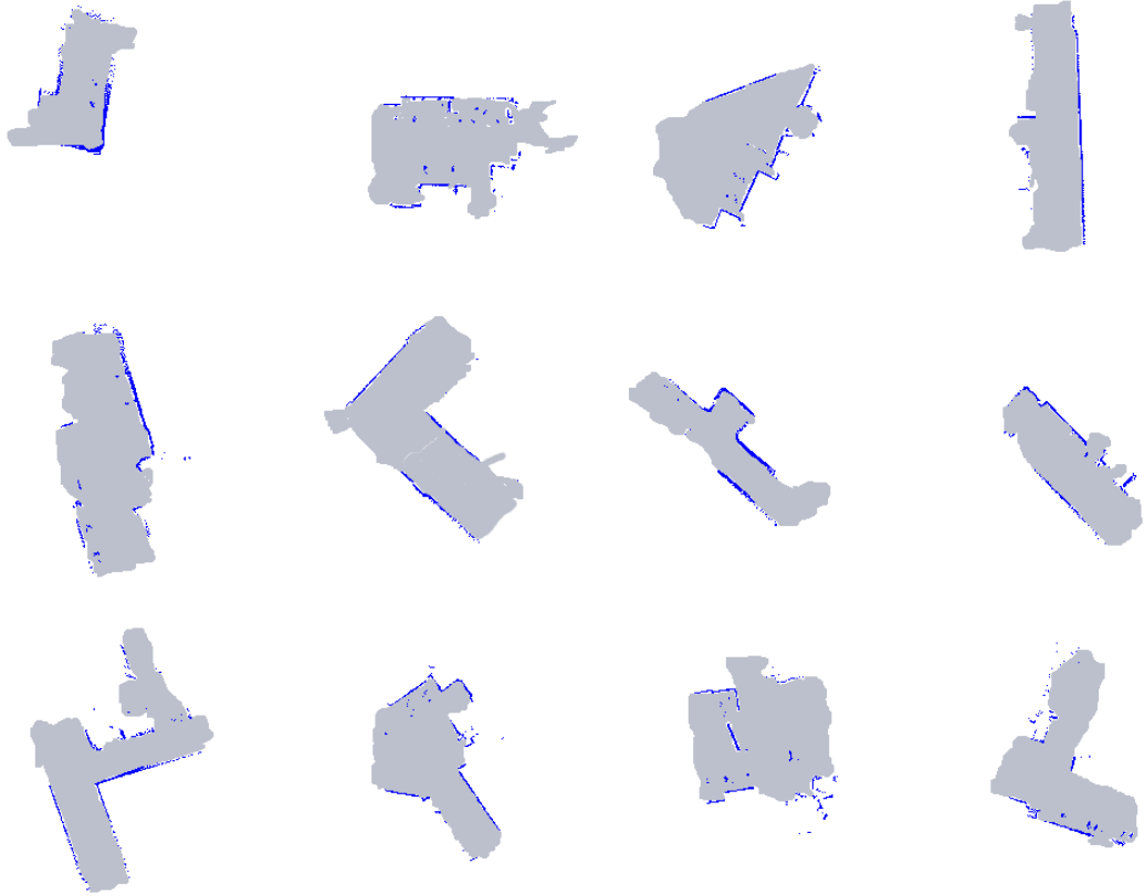
Figure 48: Scan measurements, obtained by concatenating scans from around landmark locations, used by the RBPF algorithm.
