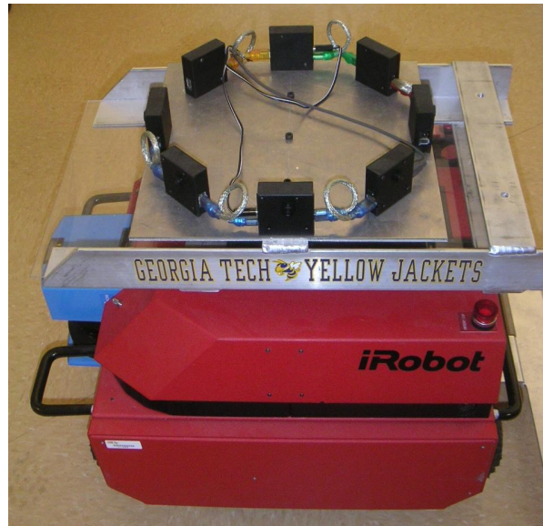
Figure 8: ATRV-mini robot with eight camera rig and forward-facing laser scanner used in experiments.
