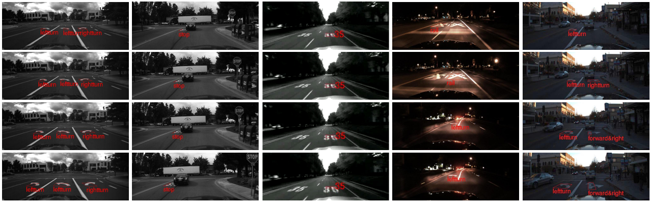
Fig. 7. Examples of road sign detection and recognition results (labeled in red) under different condition: multiple signs in cloudy weather(1st column), with occlusion in cloudy weather (2nd column), with motion blur in sunny weather (3rd column), during night (4th column), and in twilight (5th column). Night and twilight results are shown in color just to illustrate the lighting conditions better.
