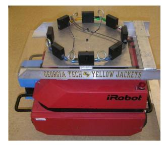
Fig. 1. The camera rig mounted on the robot used to obtain panoramic images
